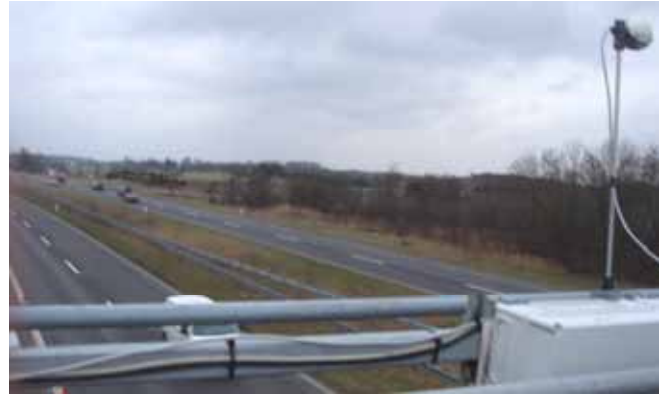
Installing the sensor is quick and easy and can be done on existing structures (e.g. VMS panels).
