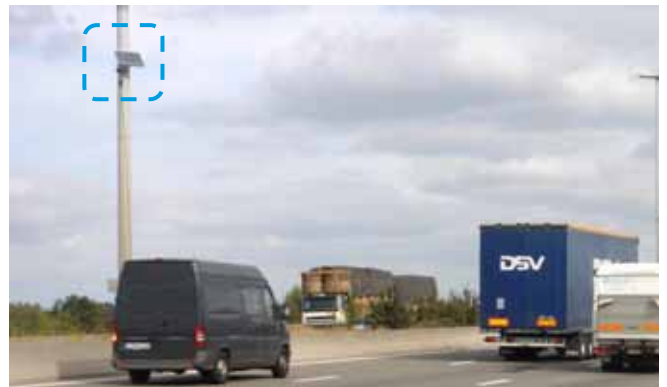
Collect-R x-stream can be powered by solar panels and used as a stand-alone queue detection system on the highway.
