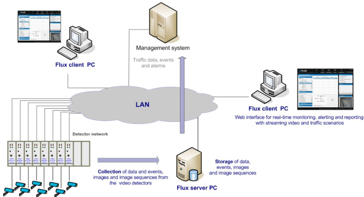
Flux is designed to handle any type of Traficon detector. Not only VIP modules can be connected to Flux but also integrated sensors like TrafiCam x-stream and Collect-R. Depending on the type of application it is even possible to combine both detectors in one system.
