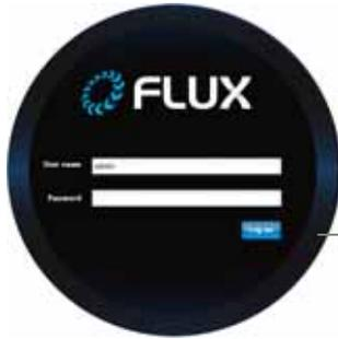
The client of Flux is a web-based application. This means users only need a web-browser installed on their PC that is connected to the network of the video detection system to access the traffic management system.
