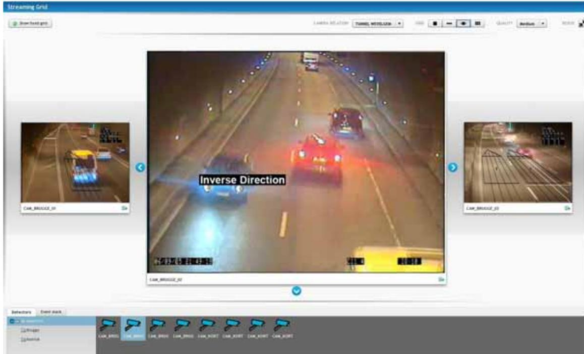
Via the streaming grid mode, and its underlying Imux streaming video server, real-time video can be viewed from several cameras simultaneously. This allows the user to have a perfect overview of different consecutive cameras.
