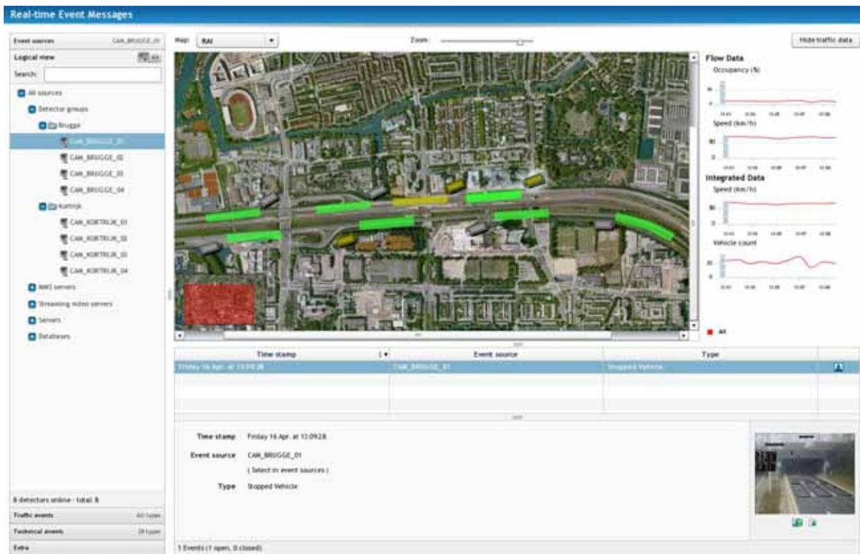
Flux enables real-time monitoring of events and real time traffic data. Traffic and technical events are automatically visualized and documented with their status, a camera image, all event info and an incident movie.
