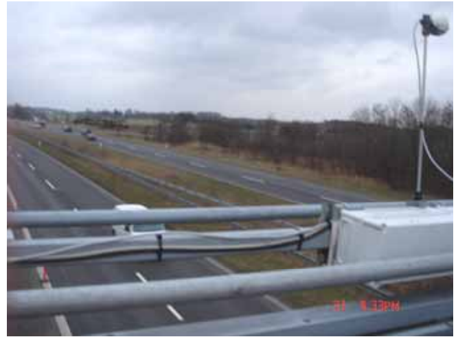
The Collect-R installed on existing structures (e.g. VMS panels).
